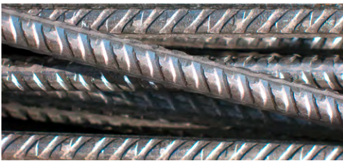
Ribbed B500 reinforcing bar on the construction site.
